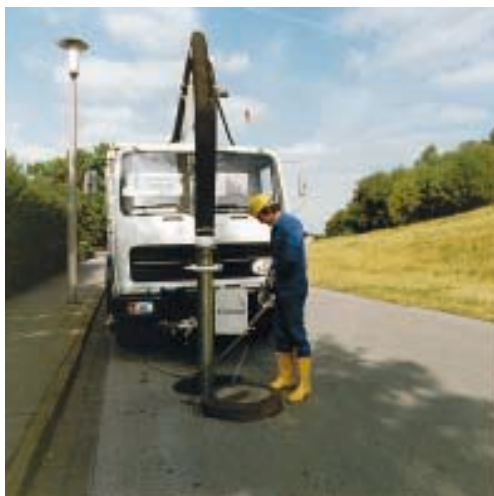
Combined suction-cleaning vehicle for sewer cleaning with reel, high-pressure cleaning nozzle and suction hose
