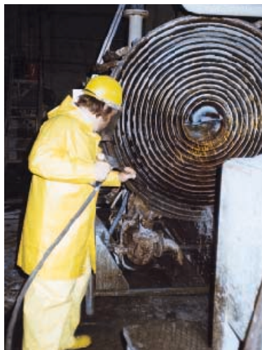
Filter cleaning in the gas concrete production
