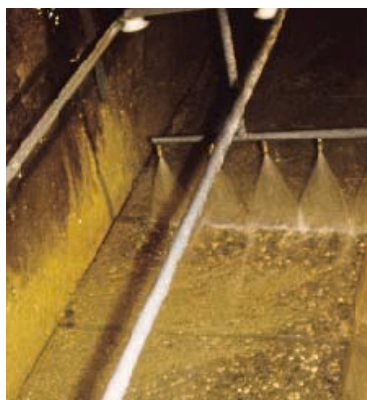
Removal of accretion rings in rotating kilns by water jet lances
