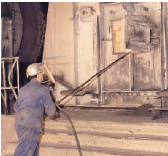
Removal of accretion rings in rotating kilns by water jet lances
