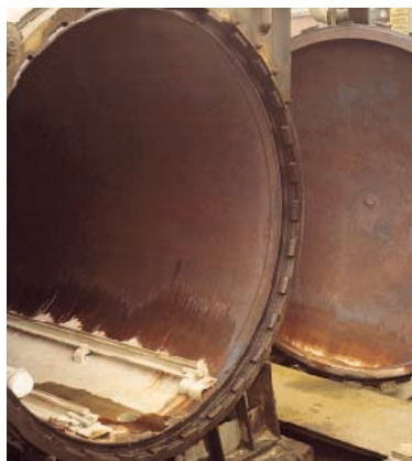
Deposit removal from lime-malm-brick tempering vessels
