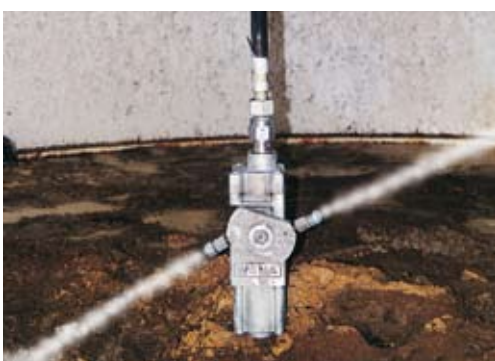
Cleaning system TankMaster® 1250 in action
